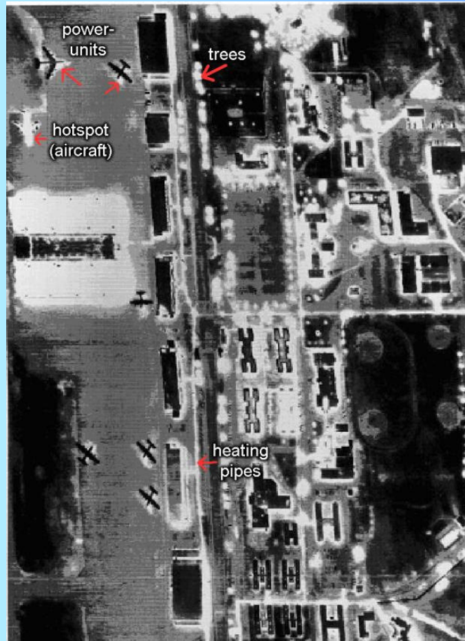
Photo: Thermal infrared line scanner image of an airport taken at night. Notice the “hot” buried heating lines and trees along the roadsides. Warm auxiliary power units can be seen near some of the aircraft. One aircraft in the upper left corner appears anomalously warm. It might have been parked in the nearby hangar not long before the image was taken. Photo: Courtesy of Intera-Kenting, Ottawa.
