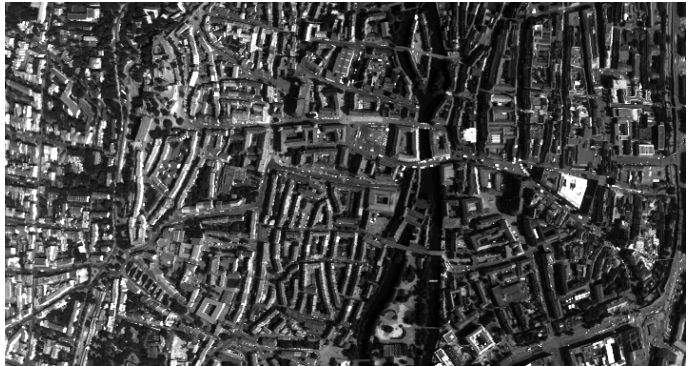
Fig. 1: Sample of the image data (about 10% of the subset 'densely populated area') at a wavelength of 0.66 \mu\text{m} , histogram equalized. Flight direction is from top to bottom, scanning direction from left to right. The sun illuminates the scene from the right. The area in backscatter direction (left) is brighter than the area in forward scatter direction (right).
