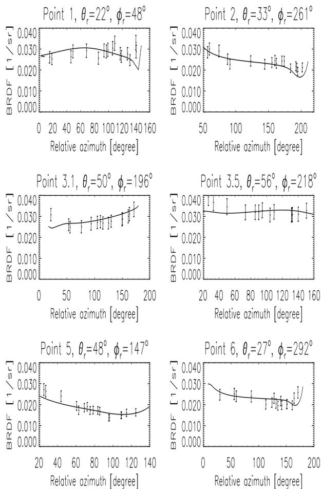
Fig. 3: Measured data (with error bars) of the BRDF from the roof in fig. 1 and fitted model (solid line) at a wavelength of 900 nm as a function of relative azimuth angle. Note that the incident zenith angle is NOT constant in these plots.  $\theta_r$  = zenith angle of reflection,  $\phi_r$  = azimuth angle of reflection,  $\phi_r = 0^\circ$  or  $\phi_r = 180^\circ$  are 'parallel to the cosine crest' (no masking from the cosine shape for these angles).
