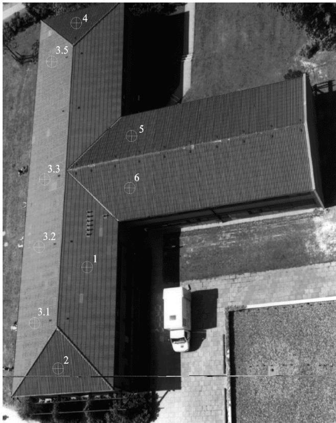
Fig.1: Investigated roof with measured points, picture taken from sensor position. The inclination of the roof surface normal to nadir is  $15^\circ$ .
