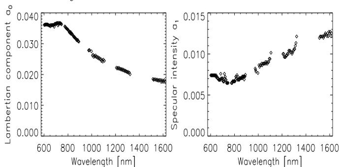
Fig. 2: Fitting  $a_0 + a_1 \times \text{Shape}_{\text{Specular}}$  as BRDF of the surface patches yields the above coefficients.  $a_0$  (plot on the left) drops by half from 610 to 1600 nm,  $a_1$  (plot on the right) doubles from 610 to 1600 nm. Wavelengths of high atmospheric absorption are not shown.
