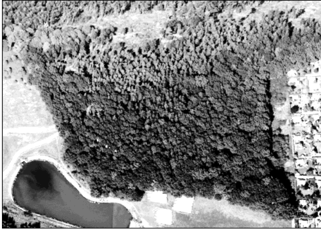
Fig. 1: Image of the Daedalus AADS 1268 airborne scanner, taken Aug. 21. 1991. A detail of the landscape south of the airport of Nürnberg (FRG) is shown in channel Daedalus 3 ( 0.52 - 0.60\mu m = TM channel 2, contrast enhanced). A small lake can be seen adjacent to a forest stand.
