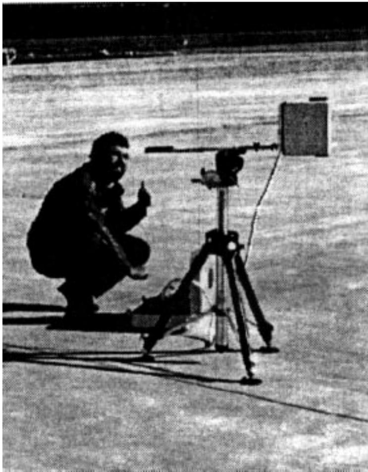
Fig. 2: The IRIS spectroradiometer (DRL)
