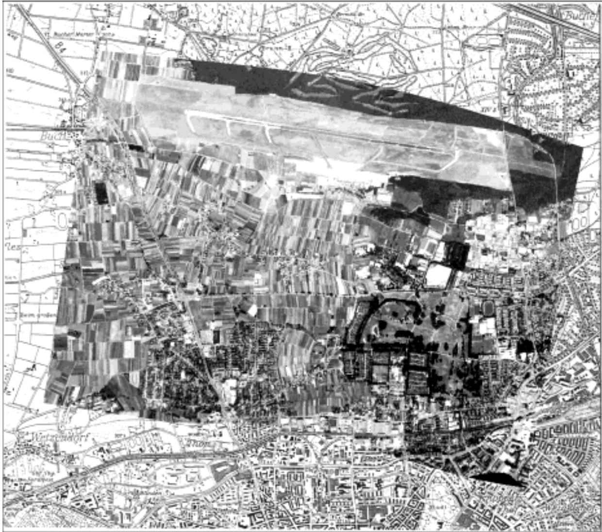
Figure 2: The geocoded image overlaid onto a map of scale 1 : 25 000, using AKIMA interpolation.
