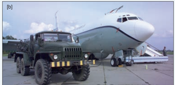
Fig. 5 (a) - A Boeing OC-135B Open Skies observation aircraft in flight. (b) - A Boeing OC-135B aircraft being prepared for flight - the "canoe" or bulge on the underside of the fuselage behind the front wheel of the aircraft undercarriage houses the SAR antenna. However the radome and antenna have since been removed from the aircraft. (Source: DTRA)
