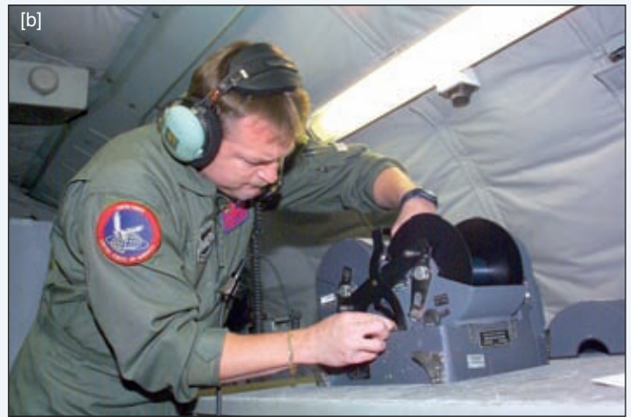
Fig. 4 - A U.S. Open Skies team in action with (a) an operator working at an imaging control station; and (b) a film magazine being changed - on-board the Boeing OC-135B aircraft - and (c) the inspection of a processed film being carried out at the Open Skies Media Processing Facility (OSMPF) in Dayton, Ohio. (Source: OSMPF)
