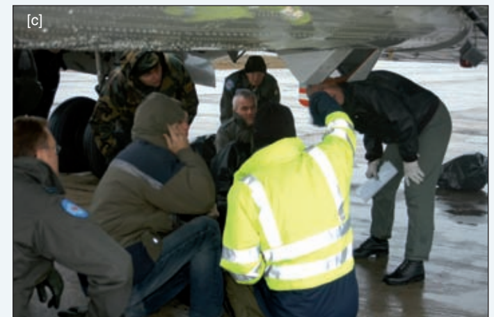
(c) - The pre-flight inspection of the underside of the Andover aircraft being carried out in Lithuania - note the camera lens protruding just below the belly of the aircraft. (Source: U.K. Open Skies Unit)
