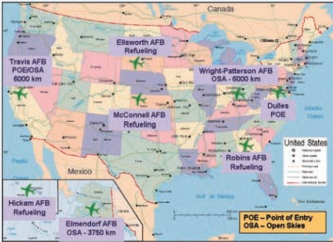
Fig. 2 - In the U.S.A., several airfields are designated for use by Open Skies observation aircraft. There are two Points of Entry (POEs) - in Washington, D.C. and California; three Open Skies Airfields (OSAs) where observation flights can start and finish; and four airfields where refuelling can take place. (Source: DTRA)
