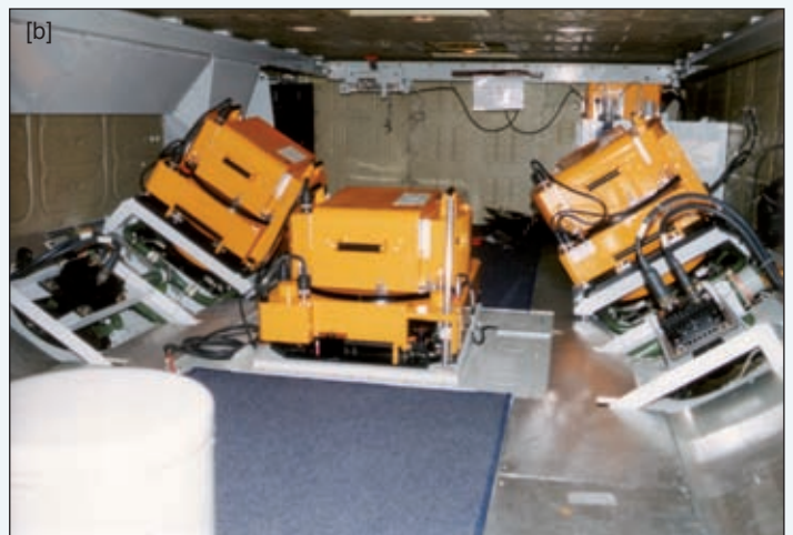
Fig. 3 (b) - The three Zeiss Jena LMK photogrammetric film cameras and three Zeiss VOS-60 video cameras (pushbroom scanners) mounted in the German Tupolev Tu-154M aircraft. (Source: IGI)
